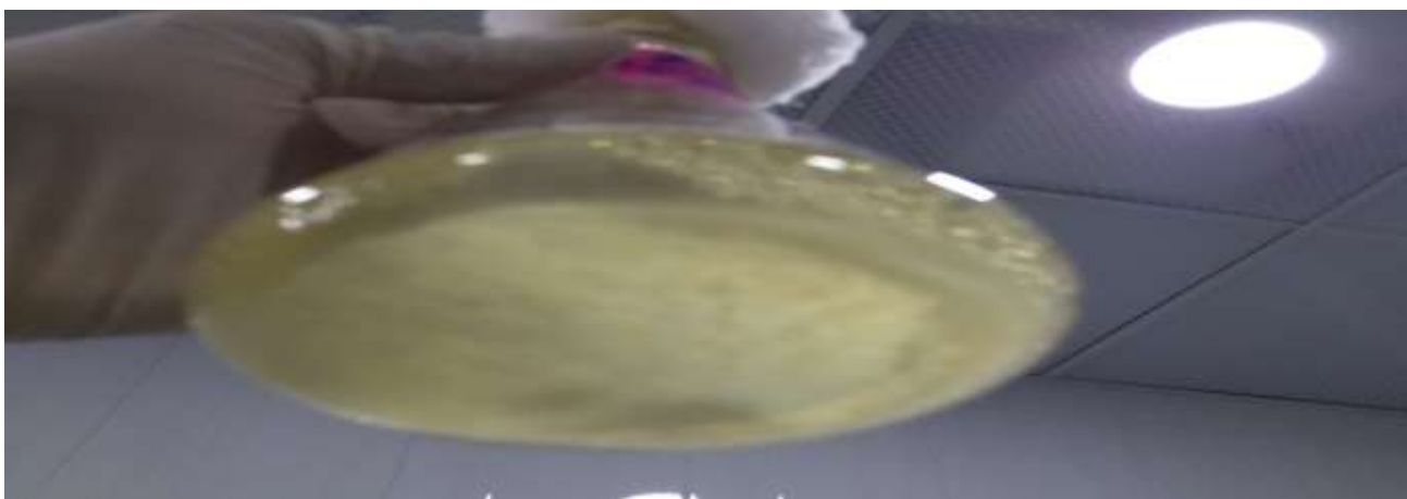
Fig.1: Precipitated of biologically ZnO NPs at the bottom of flask
