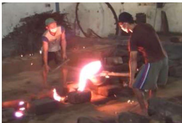
Figure 2: Two-operator Ladle-Kowi with capacity of 50 kg liquid steel
