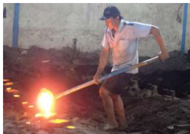
Figure 1: One-operator ladle-kowi with capacity of 15 kg liquid steel
