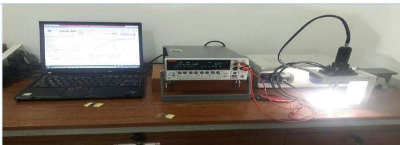
Fig. 2: A device for measuring the electrical properties of solar cells
