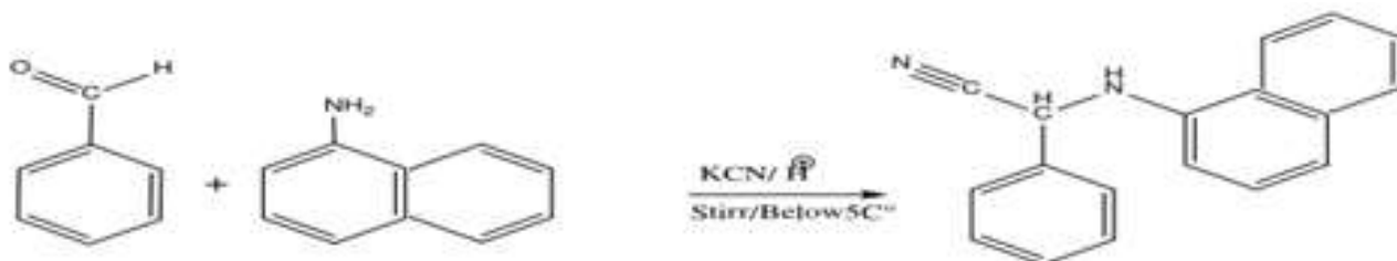
Benzaldehyde 1-Naphthylamine 2-phenyl-2-(1-Naphthylamine) acetonitrile ( L_2 )
