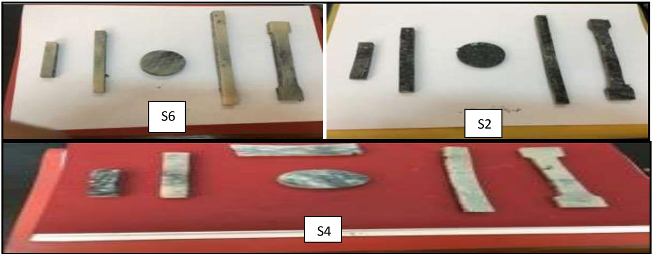
Fig. 1: Molds for new hyper- woven – micro composite material at different weight ratios from woven glass and carbon fibers
