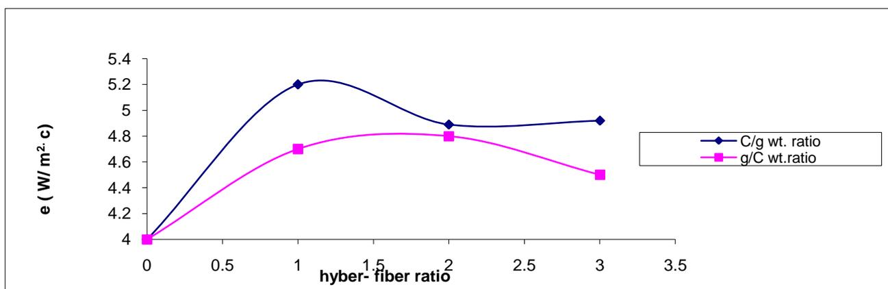
Fig.16: Shows the thermal expansion of different additive weight ratio of hyper glass and carbon fiber on values of thermal expansion for the new hyper composite
