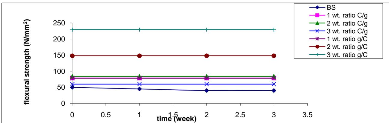
Fig.11: Shows the aging resistance (50°C and 21 day) of different additive weight ratio of hyper glass and carbon fiber on values of flexural strength for the new hyper composite
