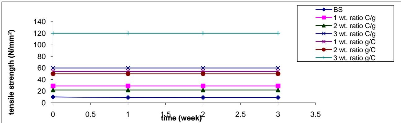
Fig. 10: Shows the aging resistance (50°C and 21 day) of different additive weight ratio of hyper glass and carbon fiber on values of tensile strength for the new hyper composite
