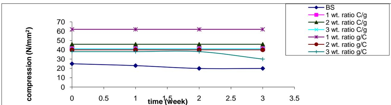
Fig.12: Shows the aging resistance (50°C and 21 day) of different additive weight ratio of hyper glass and carbon fiber on values of compression resistance for the new hyper composite
