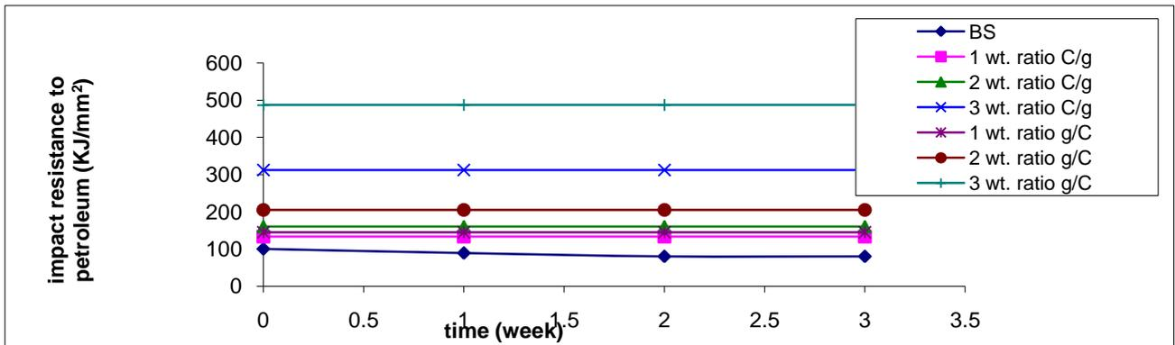
Fig. 8: Shows the aging resistance (50°C and 21 day) of different additive weight ratio of hyper glass and carbon fiber on values of impact strength for the new hyper composite
