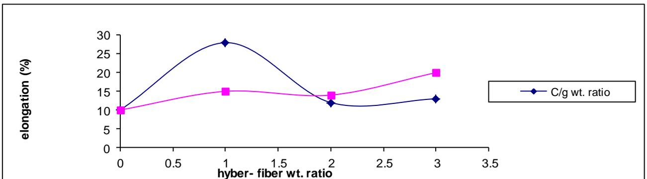
Fig. 3: Shows the effect of different additive weight ratios of hyper glass and carbon fiber on the values of elongation for the new hyper composite
