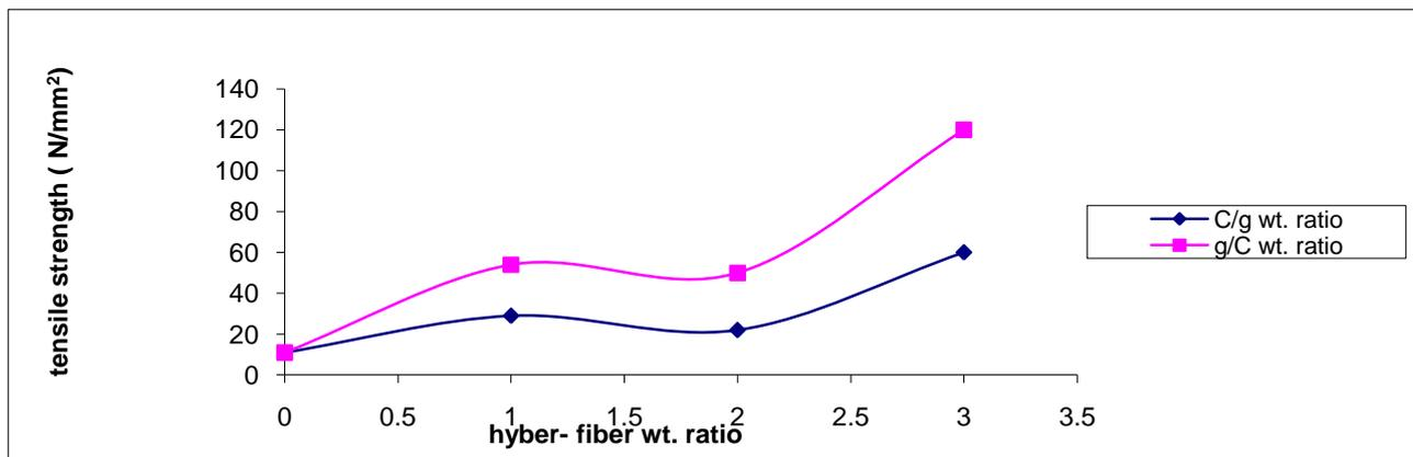
Fig. 4: Shows the effect of different additive weight ratios of hyper glass and carbon fiber on the values of tensile strength for the new hyper composite
