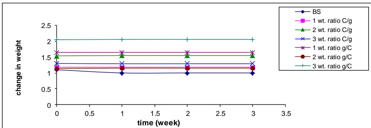
Fig.14: Shows the aging resistance (50°C and 21 day) of different additive weight ratio of hyper glass and carbon fiber on values of physic-chemical activity for the new hyper composite
