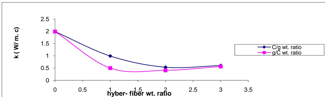
Fig.15: Shows the thermal conductivity of different additive weight ratio of hyper glass and carbon fiber on values of thermal conductivity for the new hyper composite
