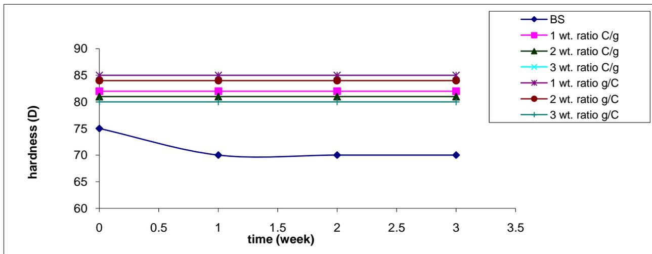
Fig.13: Shows the aging resistance (50°C and 21 day) of different additive weight ratio of hyper glass and carbon fiber on values of hardness for the new hyper composite
