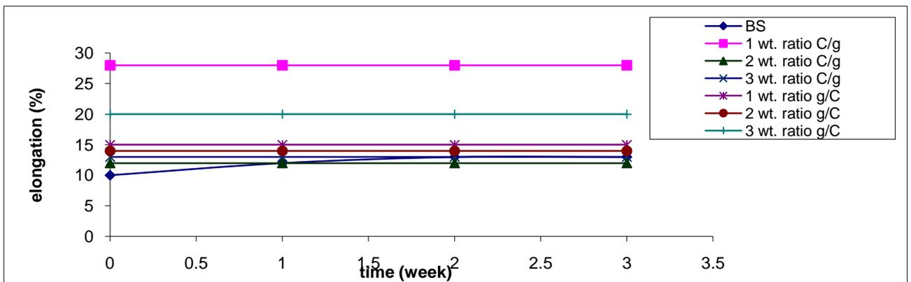
Fig. 9: Shows the aging resistance (50°C and 21 day) of different additive weight ratio of hyper glass and carbon fiber on values of elongation for the new hyper composite
