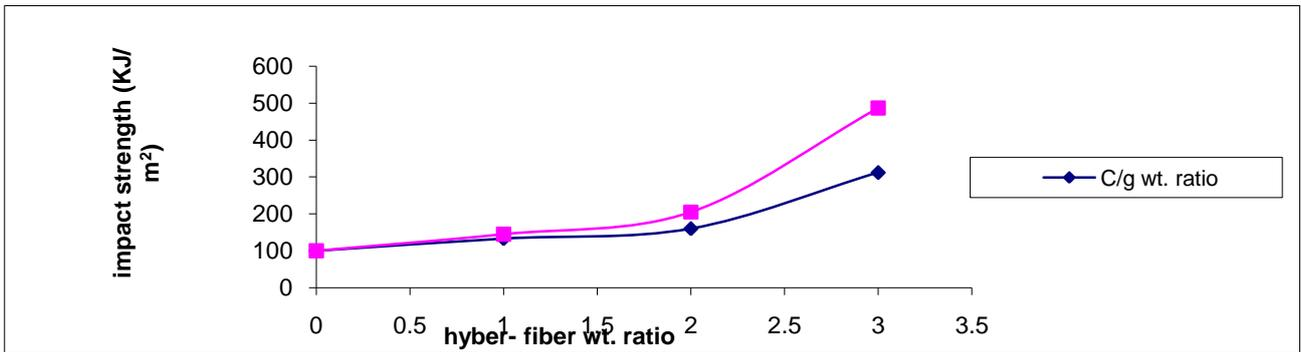
Fig. 2: Show the effect of different additive weight ratios of hyper glass and carbon fiber on the values of impact strength for the new hyper composite
