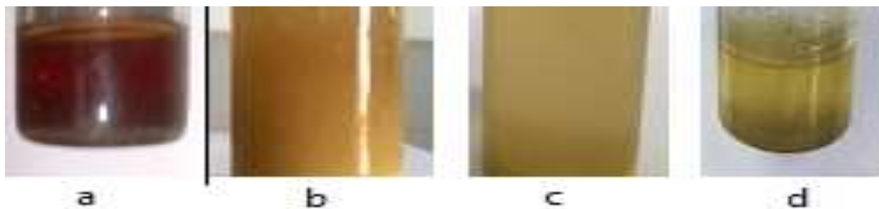
Figure 1: Optical photograph of (a) AlCl 3 -urea, (b) AlCl 3 -acetamide, (c) AlCl 3 -thiourea and (d) AlCl 3 -thioacetamide ionic liquids
