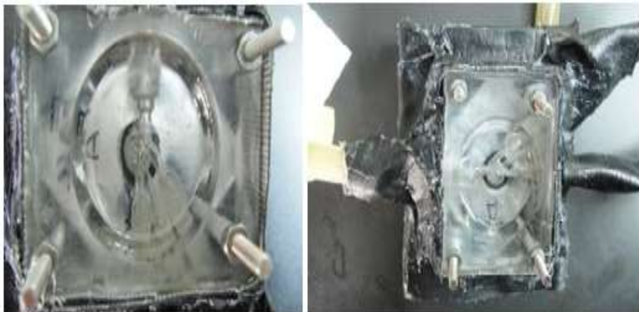
Figure No.2: A specially designed flow chemiluminescence and fluorescence cell consists of three inlets are arranged two of them are at same level while the third one is at a lower level in the cell
