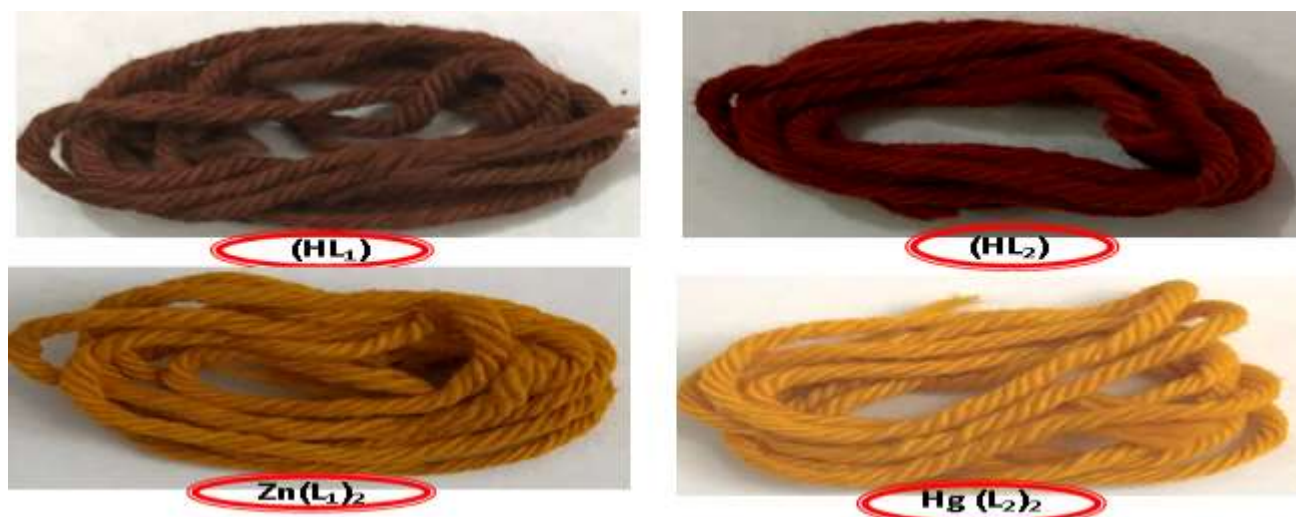
Figure 8: Samples the textiles dyeing for azo ligands and metal chelates
