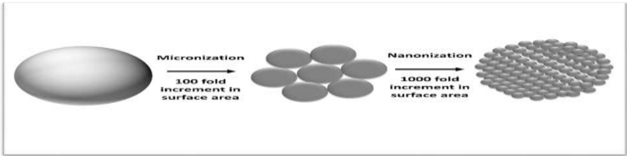
Fig. 2: A diagrammatic representation of nanonization mechanism
