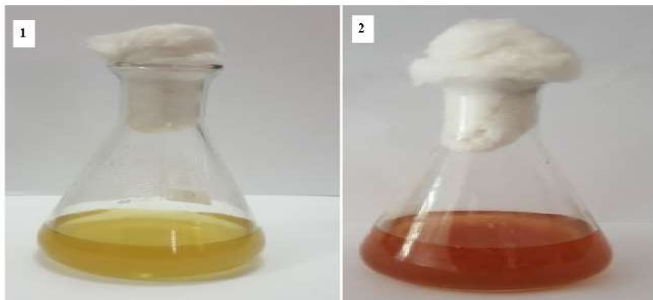
Fig.1: Ag nanoparticles synthesis by plant extract, (1) plant extract (2) extract with AgNO 3 (Ag nanoparticles)
