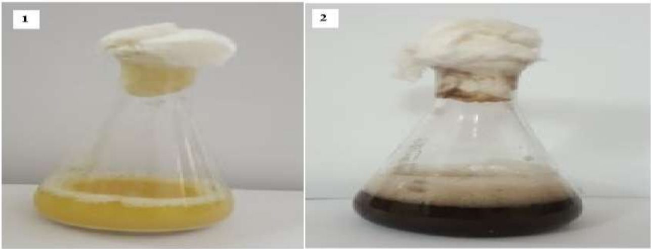
Fig.2: Ag nanoparticles synthesis by plant Extract, (1) filter of fungus (2) filter with AgNO 3 (Ag nanoparticles)
