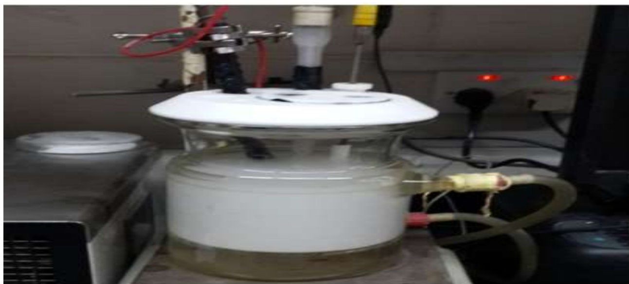
Fig. 2: The electrochemical cell for corrosion measurement of carbon steel reinforcing bar in simulates concrete solution
