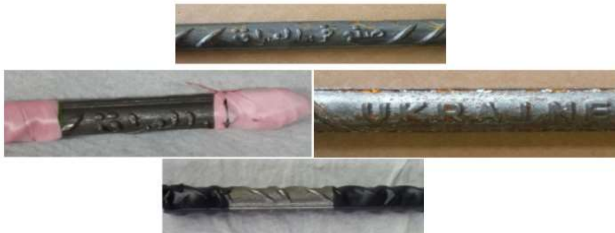
Fig.1: Preparation of the Carbon steel reinforcing bars used in this study
