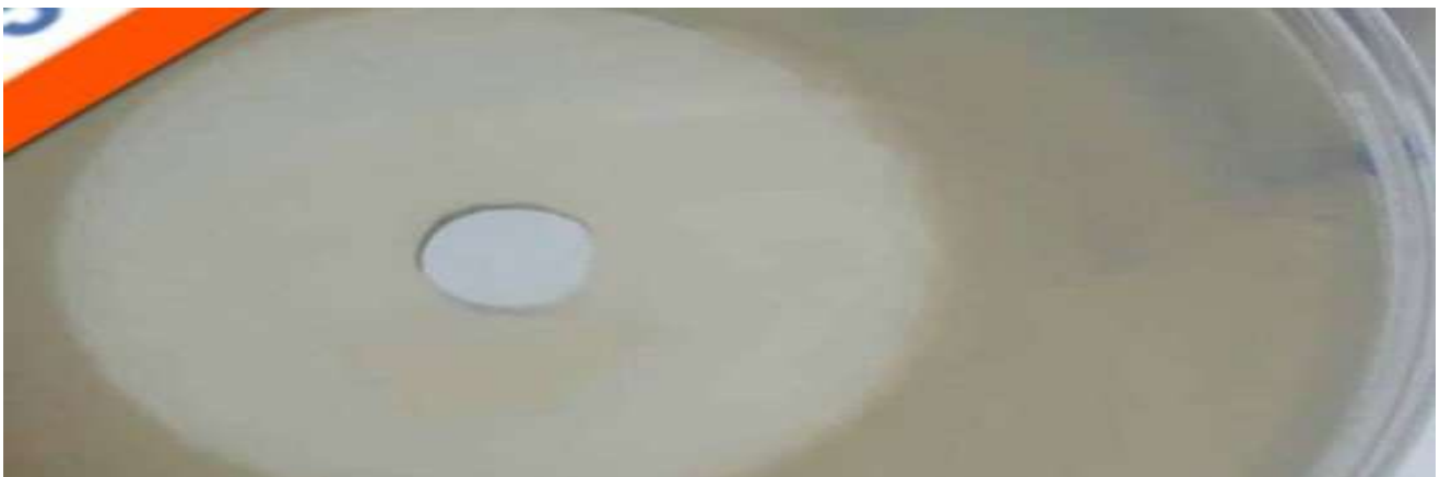
Fig. 5b :( 4%wt. MgO) Image of the bacterial colony using polymer-nanoparticles composites as an anti-bacterial
