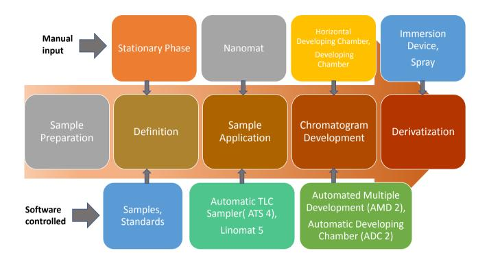
Fig. 1: Flowchart of a typical HPTLC process [8]
